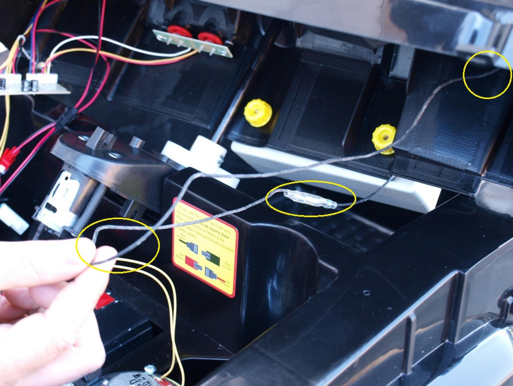
For the speaker, connect the red and black wires to the speaker terminals. For the motor, connect the red, black and green wires to the motor terminals. Make sure the connectors to the motor are connected in the correct polarity.
