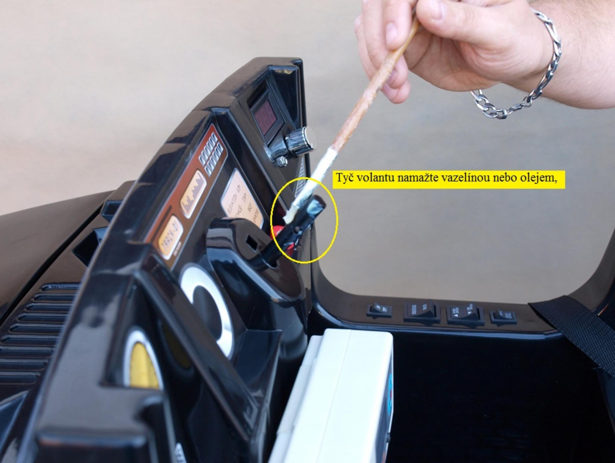
A close-up photograph of a person's hand applying grease to the steering column shaft of a motorcycle. The person is wearing a silver chain bracelet. The steering column is black plastic with various controls and labels. A yellow circle highlights the point where the grease is being applied. The background is a plain, light-colored surface.
